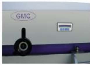
German SIKO Power Back Gauge Digital and Micro-adjustment
